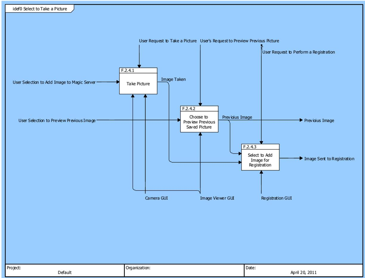
Figure 23 Select to Take a Picture (IDEF0 Diagram)
